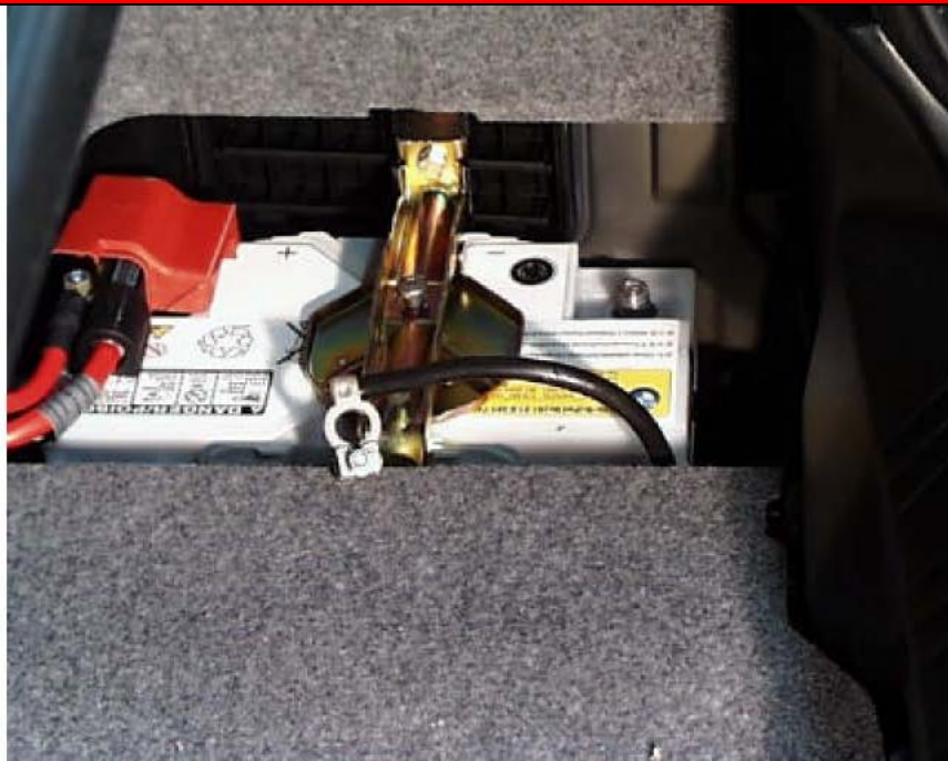
Figure 1 Disconnect the Negative terminal on the battery.
